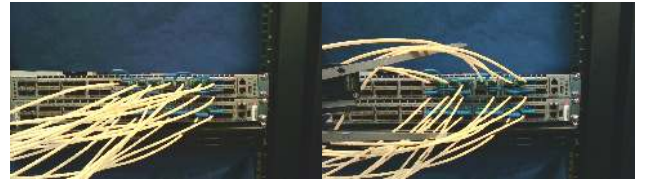
Fig. 8: Segmentation masks imposed on the camera image before and after cable parting.
