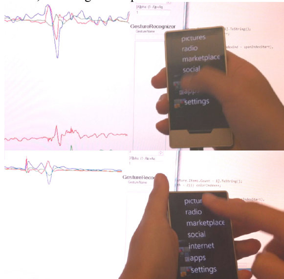
Fig. 5. Sensor traces from a three-axis gyroscope and accelerometer for one-handed scrolling with the thumb (top) versus two-handed scrolling with the index finger (bottom). See also video.
