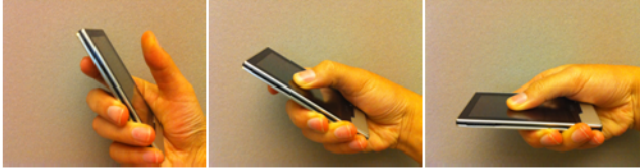
Fig. 1. Tilt-to-Zoom: No zooming occurs while the device is held normally (left). Touching the screen enters the zooming mode (middle). Zooming is then mapped to the change in tilt angle (right).
