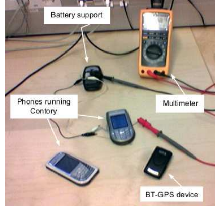
Fig. 3. Power measurements testbed setup
