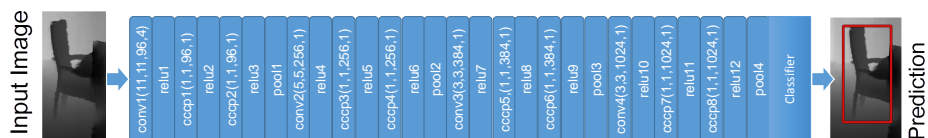
Fig. 4. Shallow ConvNet model architecture. This figure presents our inference process during inference time. We adapted successful network configuration described in [28] for this task.
